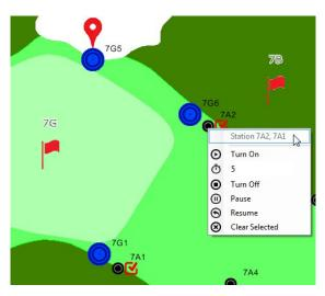
Should a user want to turn off the partial area manual irrigation it is easiest to select the area marker and choose the 'Turn Off' option for each area separately.
